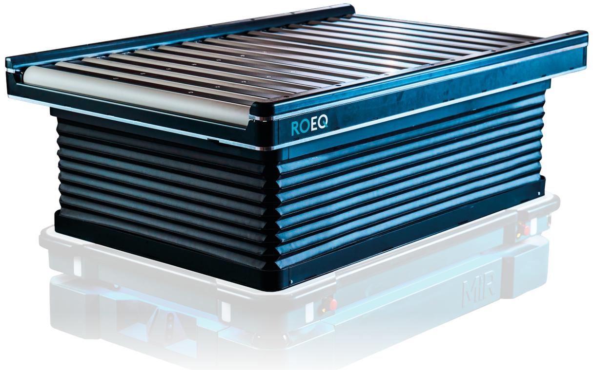
The ROEQ TR500 Auto allows you to use your MiR500, MiR600, MiR1000 and MiR1350 robots to transfer heavy goods between conveyor stations at different heights. It has a built-in scissor mechanism for automatic height adjustments. Using the ROEQ Assist software tool for set up, you can easily program the pick-up and delivery points in the MiR GUI. With a large stroke – 240mm/9.4” – it gives you the flexibility to adjust to your existing setup.
